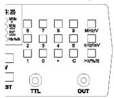
Among them, there are 10 number keys: "." Decimal point key, "C" backspace key, "MHz/V" MHz or V unit key, "KHz/mV" KHz or mV unit key, "Hz/%/S" Hz unit key or modulation depth % or S unit key.
